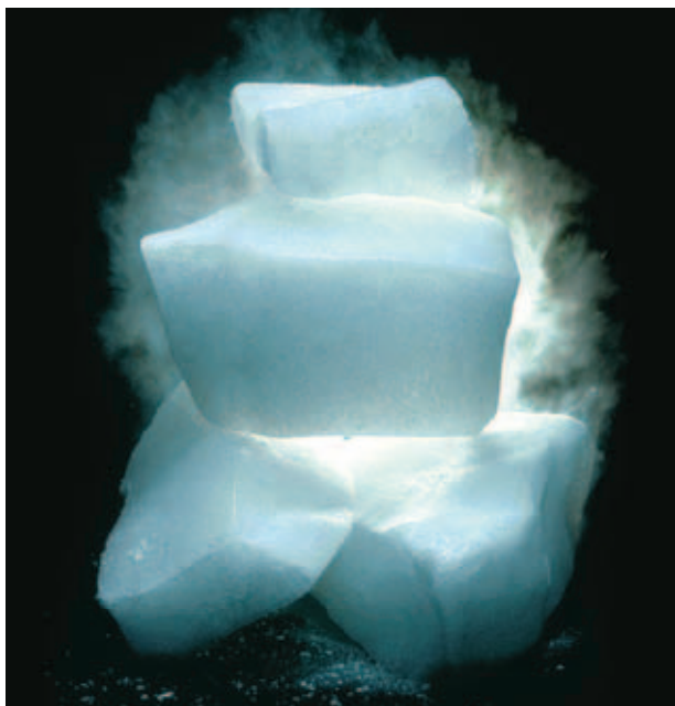
Figure 6 Dry ice changes directly from a solid to a gas. This change of state is called sublimation.
